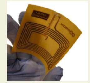
Figure 2: The first flexible sensor prototype developed by Sabanci University and Kordsa in April 2019.
