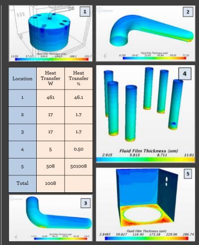
*Figure 7: Heat transfer rate for components of the heating box* (Design 2)
