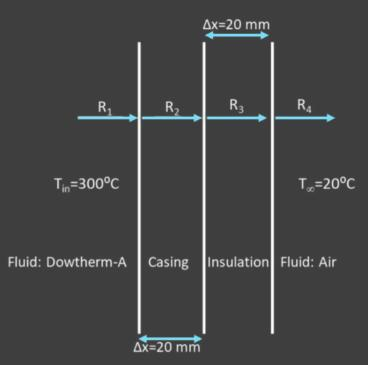
Figure 3: Resistances in the casing and insulation of the heating box system
