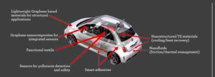
Figure 2. Graphene-based applications in a vehicle<sup>3</sup>
