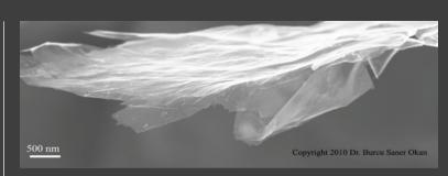
*Figure 1. Electron microscopy image of graphene sheets*
