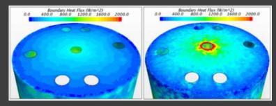
Figure 6: Heat flux distribution comparison of the top surfaces of the solidification chambers in Designs 1 & 2
