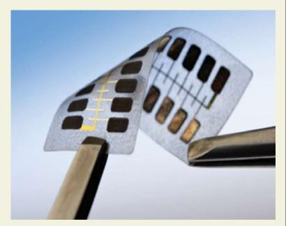
*Figure 4: A sample of flexible electronics*
