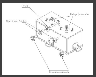
Figure 1: Schematic figure of a heating box (Dow-box)
